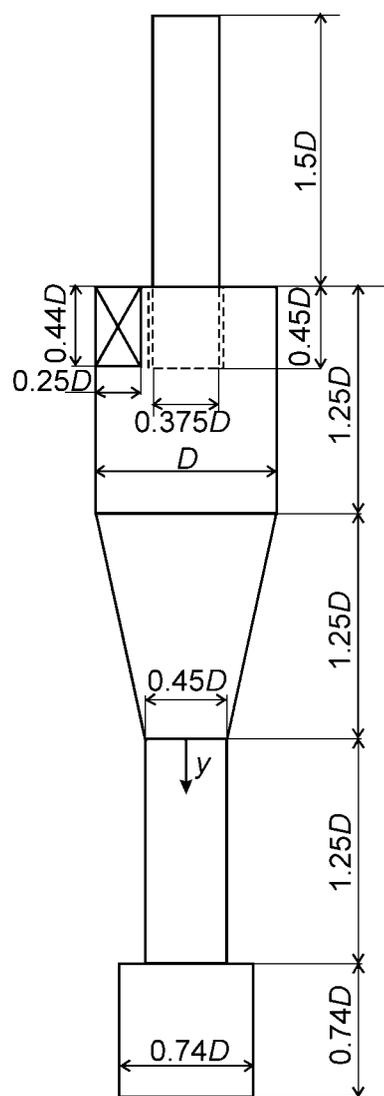
**Figure 1. Cyclone geometry due to Obermair et al.**<sup>18</sup>
