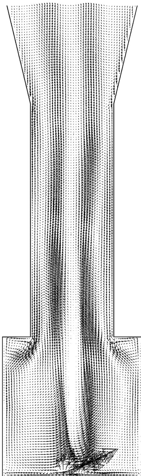
Figure 4. Particle flux vectors (local particle velocity times particle concentration) in the lower part of the Obermair et al.<sup>17,18</sup> cyclone for a two-way coupled, two-phase simulation with particles of 5.4  $\mu\text{m}$ .
