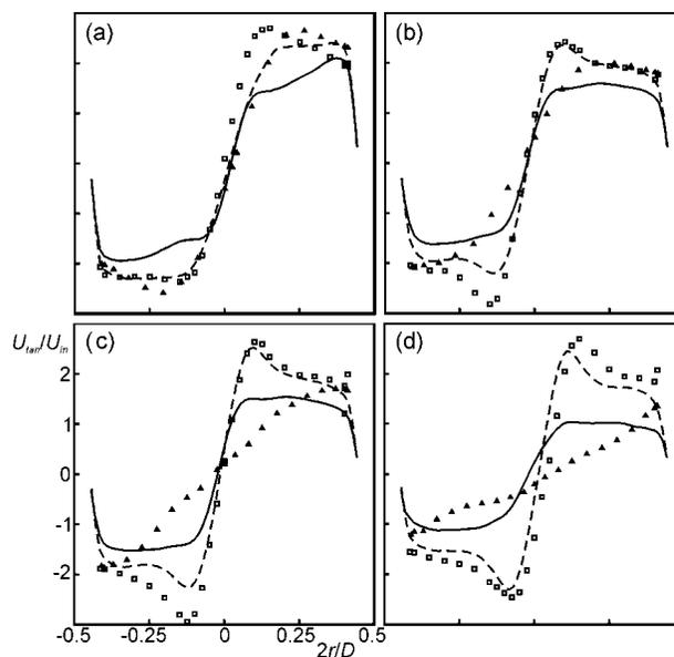
**Figure 3. Radial profiles of the tangential gas velocity for various axial positions (chosen according to the experimental data in Figure 8 of Obermair et al.<sup>17</sup>) in the downcomer.**
