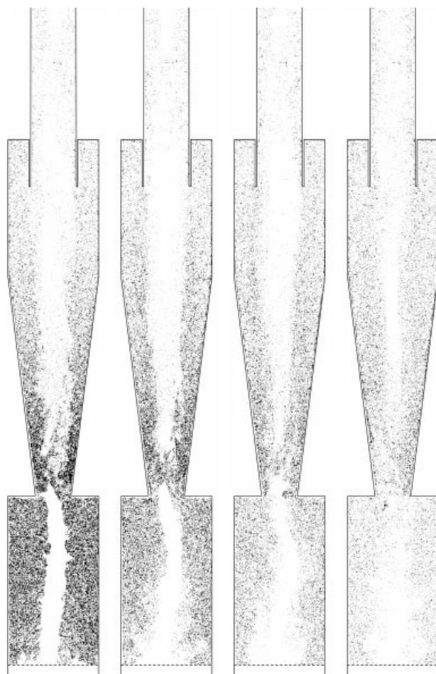
Figure 8. Instantaneous realizations of the particles with  $Stk = 2.3 \cdot 10^{-3}$  in vertical slice, with thickness of  $0.02D$  through the center of the cyclone (the  $xy$ -plane) in (from left to right) a one-way coupled simulation, and two-way coupled simulations with mass-loading 0.00625, 0.025, and 0.1, respectively.
