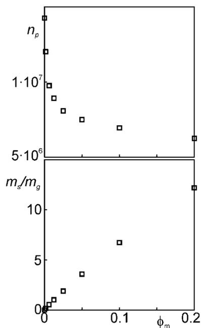
**Figure 9.** Total number of parcels (top), and total solids mass (normalized with the total mass of gas) inside the Stairmand cyclone under steady-state conditions as a function of the mass loading (zero mass loading: one-way coupled,  $\phi_m > 0$ : two-way coupled).
