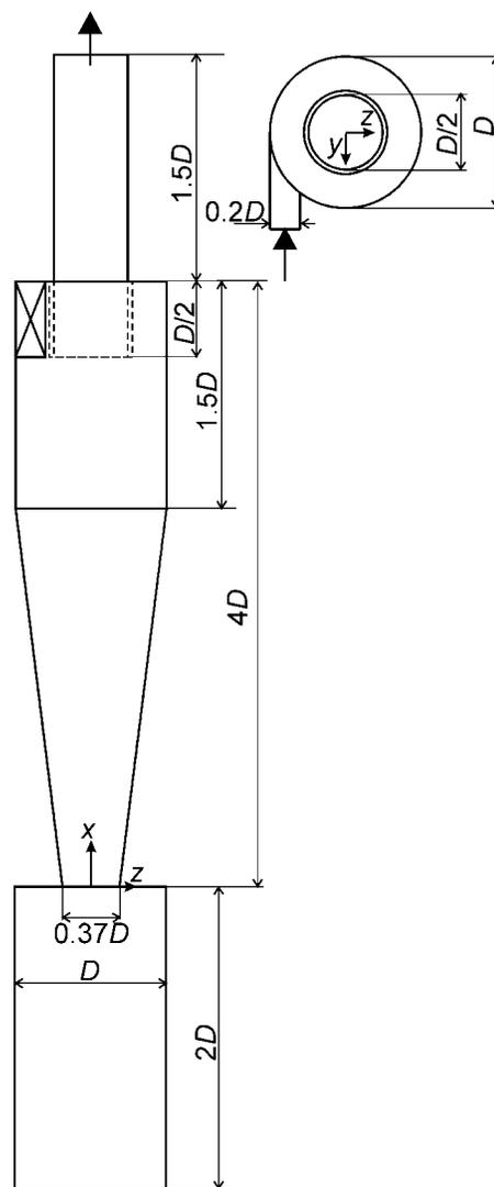
Figure 5. Flow geometry and coordinate system of the Stairmand cyclone: left: side view, right: top view.
