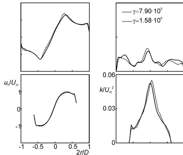
**Figure 18. Swirl and turbulent kinetic energy profiles at  $x/D = 3.25$  (top), and 1.0. Sensitivity with respect to the number of particles per parcel  $\gamma$ . Two-way coupled simulations with  $\phi_m = 0.1$  (cases 8 and 9).**
