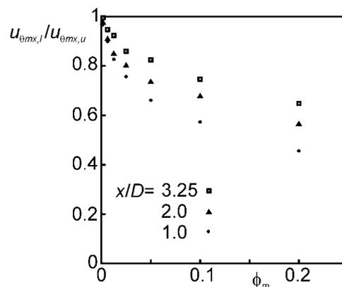
**Figure 12. Decay of the swirl velocity in terms of the ratio of the maximum swirl velocity under loaded ( $u_{\theta,max,l}$ ) and unloaded ( $u_{\theta,max,u}$ ) conditions as a function of mass loading for three axial levels in the cyclone.**
