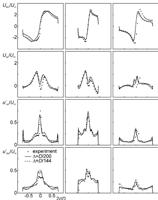
**Figure 2. Radial profiles of the tangential and axial velocity at three axial levels in the Obermair et al.<sup>17,18</sup> cyclone at  $Re = 3.4 \cdot 10^5$ .**
