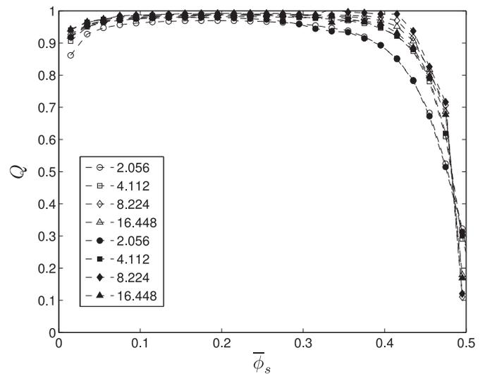
**Fig. 7.** Correction to the interphase heat transfer coefficient ( $Q$ ) as a function of the filtered solids volume fraction ( $\bar{\phi}_s$ ). Legend indicates dimensionless filter size. Open/Filled symbols correspond to a grid resolution of 1.25 mm/2.5 mm.
