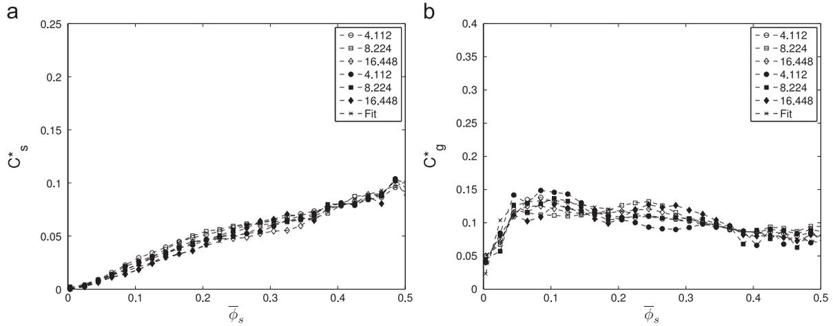
**Fig. 2.** Dimensionless filtered thermal diffusivity coefficient as a function of filtered particle volume fraction for different filter sizes. Legend indicates dimensionless filter size. Open/filled symbols correspond to a grid resolution of 1.25 mm/2.5 mm. The dashed line with 'x' marker symbol is a fit to the data. (a) particle phase and (b) gas phase.
