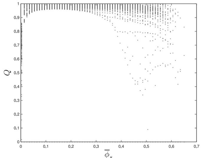
Fig. 5. Scatter plot of the correction to the interphase heat transfer coefficient,  $Q$ . Each point corresponds to a specific combination of  $\bar{\phi}_s$ ,  $|\bar{\mathbf{v}}_s - \bar{\mathbf{v}}_g|$ , and  $\hat{\Delta}$ .
