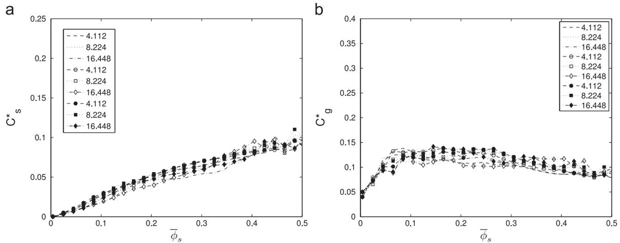
Fig. 4. Dimensionless filtered thermal diffusivity coefficient as a function of filtered particle volume fraction for different filter sizes. Dashed lines without symbols corresponds to  $e_p = 0.9$ . Open/filled symbols correspond to  $e_p = 0.85/0.95$ . (a) particle phase and (b) gas phase.
