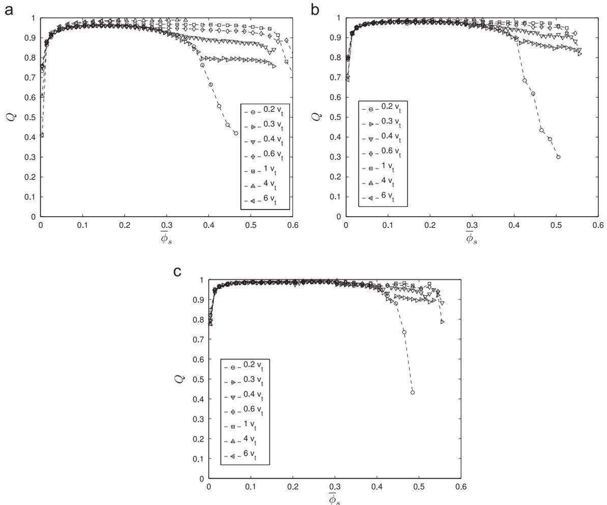
**Fig. 6.** Correction to the interphase heat transfer coefficient ( $Q$ ) as a function of the filtered particle volume fraction ( $\bar{\phi}_s$ ). Legend indicates filtered slip velocity in terms of the terminal velocity. Dimensionless filter size,  $\hat{\Delta}$ , is (a) 2.056 (1 cm), (b) 4.112 (2 cm), and (c) 8.224 (4 cm).
