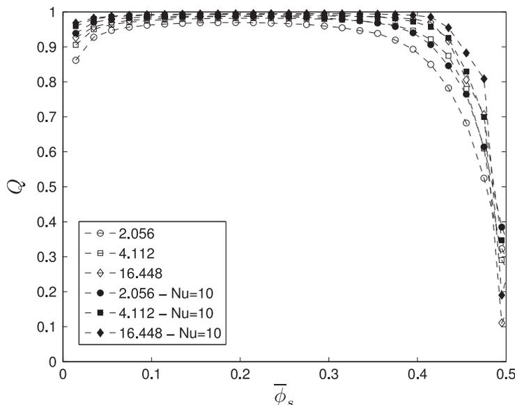
Fig. 9. Correction to the interphase heat transfer coefficient ( $Q$ ) as a function of the filtered particle volume fraction ( $\bar{\phi}_s$ ). Legend indicates dimensionless filter size. Filled symbols correspond to the case where Gunn's correlation for the Nusselt number is replaced with a constant Nusselt number value of 10.
