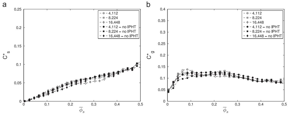
Fig. 3. Dimensionless filtered thermal diffusivity coefficient as a function of filtered particle volume fraction for different filter sizes. Legend indicates dimensionless filter size. Filled symbols correspond to the case where interphase heat transfer is not permitted. (a) particle phase and (b) gas phase.
