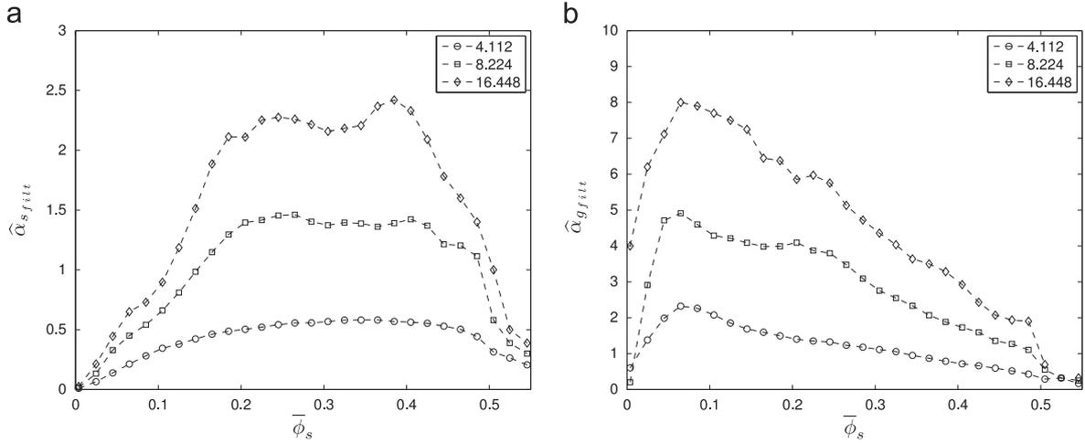
**Fig. 1.** Dimensionless filtered thermal diffusivity as a function of filtered particle volume fraction for different filter sizes. Legend indicates dimensionless filter size. (a) particle phase and (b) gas phase.
