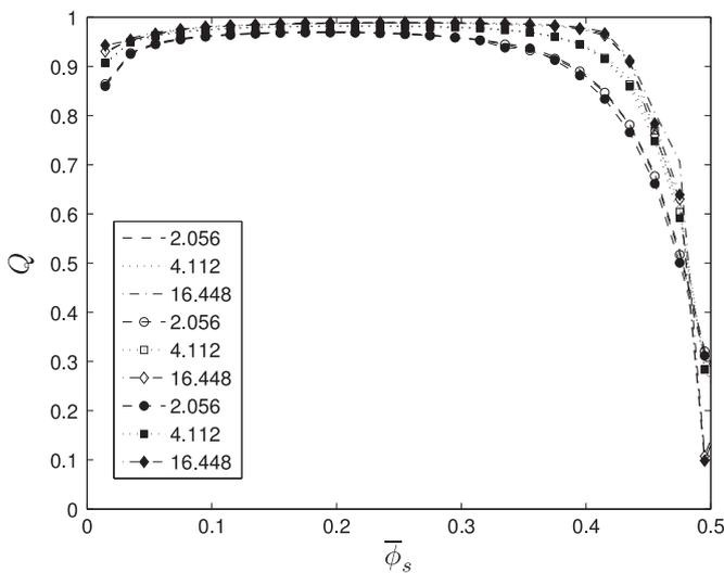
Fig. 8. Correction to the interphase heat transfer coefficient ( $Q$ ) as a function of the filtered particle volume fraction ( $\bar{\phi}_s$ ). Legend indicates dimensionless filter size. Dashed lines without symbols correspond to  $e_p = 0.9$ . Open/filled symbols correspond to  $e_p = 0.85/0.95$ .
