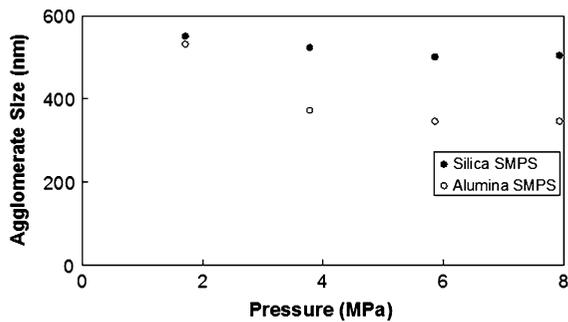
Fig. 2 Volume-weighted diameters of silica and alumina nanopowders deagglomerated (separately) through the REHPS process from various pressures. Sizes were measured with the scanning mobility particle spectrometer (range of 25–572 nm) (To et al. 2009)
