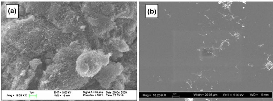
**Fig. 9** SEM images of carbon nanotubes (a) before and (b) after deagglomeration through the REHPS process. The sample was expanded from 7.93 MPa and 46
