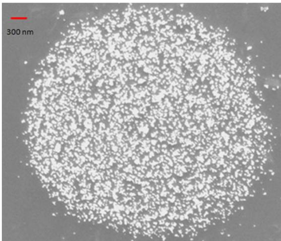
Fig. 4 SEM image of silica deagglomerated from 11.03 MPa and 45 C. It appears that dry ice precipitation during expansion from high pressures prevented effective deagglomeration
