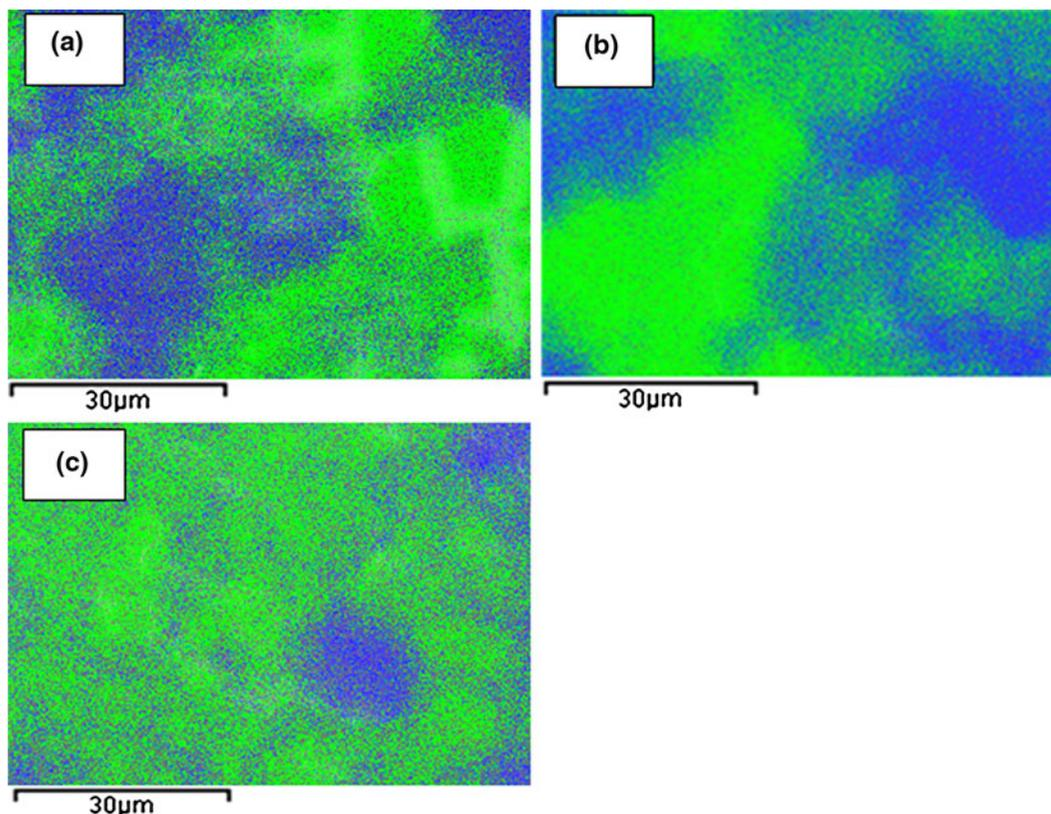
Fig. 5 Superimposed EDS scans of elemental Al (green) and Si (blue) of (a) 50:50 hand-mixed, (b) 72:28 hand-mixed, and (c) stirred premixed powders before the REHPS process. (Color figure online)
