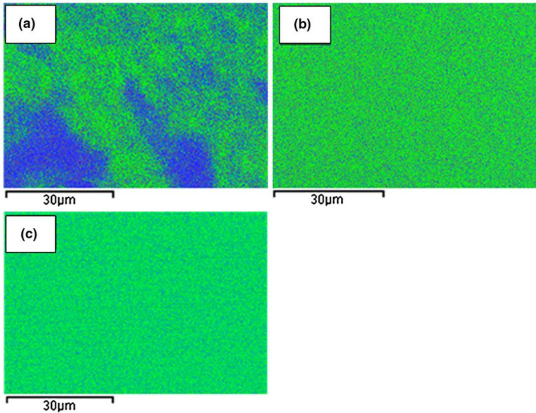
Fig. 6 Superimposed EDS scans of elemental Al (green) and Si (blue) of (a) the hand-mixed powders that remained in the expansion nozzle, (b) 1-pass, and (c) 2-pass REHPS-mixed powders. Alumina:silica weight ratio = 72:28. Sample connecting tubing between the high-pressure vessel and the expanded from 7.93 MPa and 46. (Color figure online)
