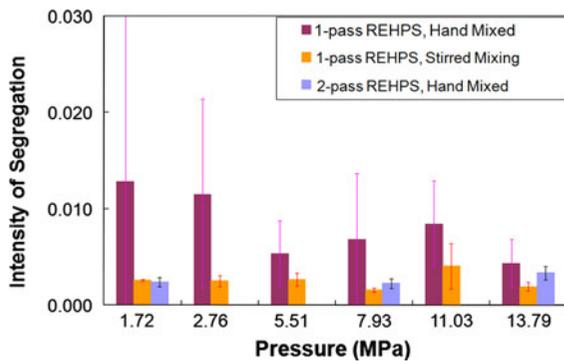
Fig. 7 IOS values for alumina/silica mixtures (50/50 wt%) expanded from different pressures through a 254- $\mu$ m nozzle. The results are shown for mixtures prepared in three different ways: hand-premixed 1-pass REHPS, hand-premixed 2-pass REHPS, and stirred-premix 1-pass REHPS. See Table 1 for more details about the mixing conditions
