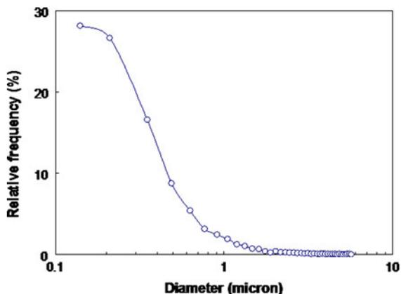
Fig. 10 Size distribution obtained through image analysis of REHPS-deagglomerated CNT
