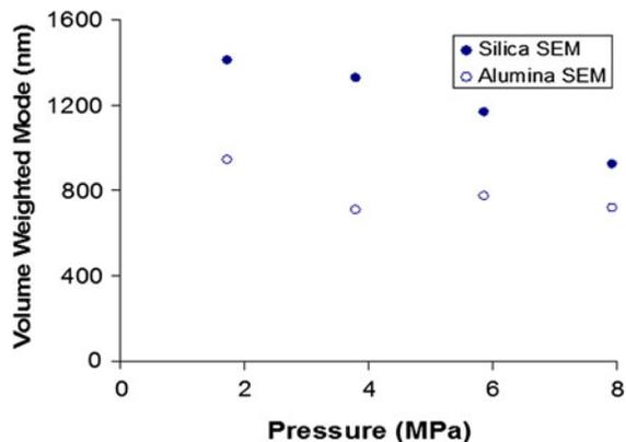
Fig. 3 Volume-weighted diameters of silica and alumina nanopowders deagglomerated (separately) through the REHPS process from various pressures. The agglomerates collected by diffusion and imaged at 33,000 with electron microscopy were analyzed to determine the sizes. Measurable sizes ranged from 40 to 3,000 nm (To et al. 2009)
