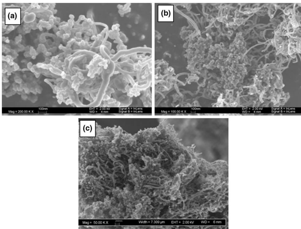
Fig. 11 Scanning electron micrographs of mixtures of carbon nanotubes and (a) silica, (b) titania, and (c) alumina nanopowders obtained through the REHPS process. Samples were expanded from 7.93 MPa and 46. Mixing at submicron scale is clearly evident. Scale bars denote 100, 100, and 200 nm for images a, b, and c, respectively
