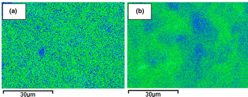
Fig. 8 Superimposed EDS scans of elemental Al (green) and Si (blue) for 1-pass REHPS through nozzles with different diameters a 508  $\mu$ m and b 1,524  $\mu$ m. The EDS elemental scan
