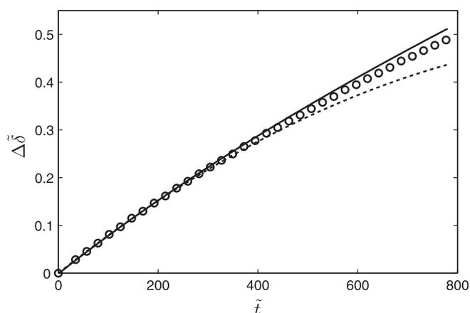
**Fig. 4.** Comparison of film growth from LB (open circles) with the two analytical models of Eq. (15) (solid line) and Eq. (19) (broken line), for  $Da_s = 288$ ,  $H_A = 8.3e-4$ ,  $\delta_0 = k_s \delta_0 / L = 4.82e-6$ ,  $x_A^s(\bar{z}, \bar{t} = 0) = 1$ .
