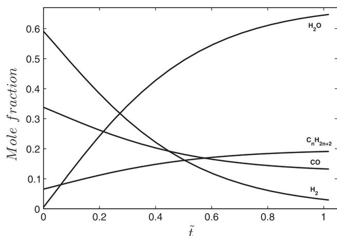
Fig. 8. Mole fractions of the four components involved in the FTS reaction vs. characteristic time.
