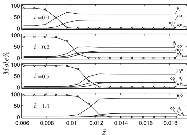
**Fig. 5.** Molar percent distribution of the four species vs. characteristic length  $\delta_0 = k_s \delta_0 / L = 4.69\text{e-}6$  at different characteristic time  $\tilde{t} = k_s^2 t / D$ .
