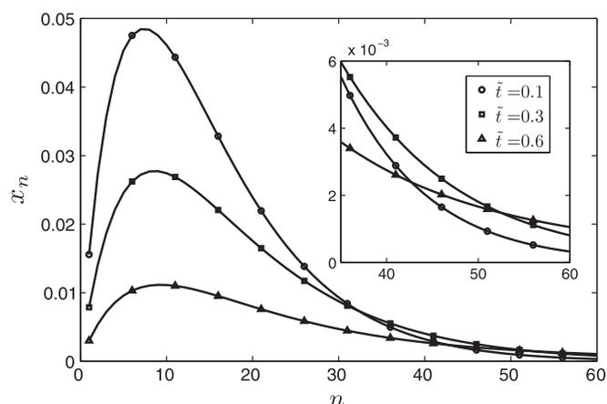
Fig. 10. Paraffin product distribution in time for the carbon chains of  $C_1$ – $C_{60}$ ; inset: zoom in the higher carbon chains.
