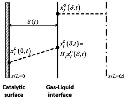
Fig. 2. schematic representation of the liquid film growth due to surface reaction (*j*: component).
