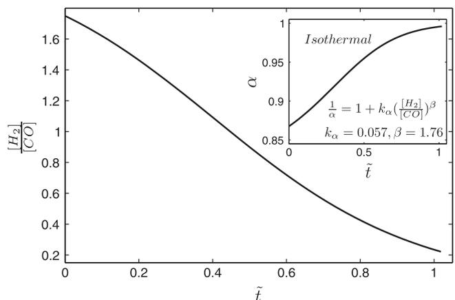
**Fig. 7.** Decrease of syngas ratio at the wall during the isothermal reaction. Inset: the increase in carbon growth probability during the reaction.
