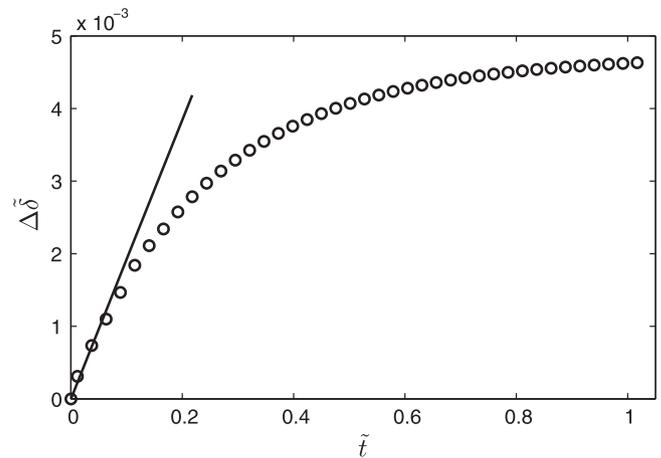
**Fig. 6.** Paraffin film growth obtained from LB simulation (circles) compared to the quasi-steady model of Eq. (15) (solid line);  $Da_s = 0.56$ ,  $H_{H_2} = 1.95\text{e-}2$ ,  $\delta_0 = k_s \delta_0 / L = 4.69\text{e-}6$ ,  $\Delta \delta = \delta - \delta_0$ .
