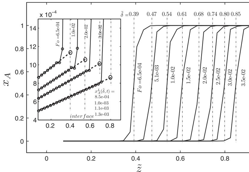
Fig. 3. Mass fraction of reactant A next to the catalytic surface at different *Fo* values. Broken lines indicate the interface locations at various *Fo*. Inset: the mass fraction linear profiles in the liquid phase and the predicted mass fraction at the interface, at various *Fo* numbers.
