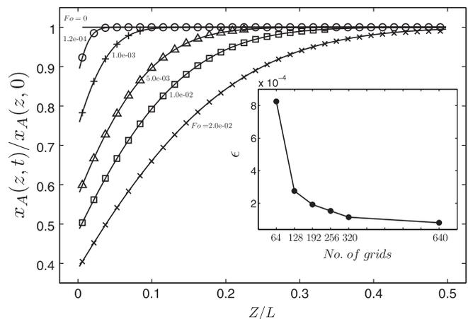
**Fig. 1.** Validation of LB model against analytical solution for a one-dimensional single-phase reaction–diffusion problem. First-order surface reaction at catalytic wall ( $z = 0$  is shown);  $Da_s = 4000$ . Bullets: LB simulation. Lines: analytical solution at various Fourier numbers. Inset: Results from a grid dependency study with the spatially and  $Fo$ -averaged relative error  $\epsilon = |x^{LB} - x^{an}|/x^{an}$ .
